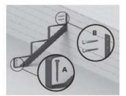
A: Attach bottom of each stringer using M10 x 50 mm coach screws\* for timber, or M10 x 60 mm Ramset™ WERCS Ankascrew™ anchors for concrete.
