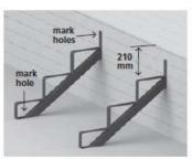
1 Determine the location of all stringers and ensure the top tread support is 210 mm down from upper deck surface. Then, for each stringer, level and mark the two fastener locations on the deck rim, and one fastener location on the lower deck surface.
