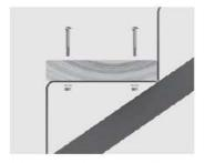
3 Install each timber tread using M8 x 60 mm cup head bolts, nuts and washers.
